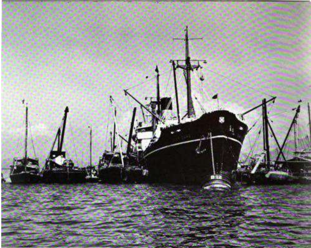
A freighter moored to a Hong Kong harbor buoy off-loads its cargo into junks and lighters. There most cargo is handled in this way, rather than by transferring it directly to piers.
