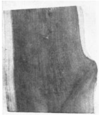
FIG. 70. Longitudinal, tangential section of yew. In this section, taken with the "grain," the annual rings appear as alternate parallel strips of dark and light wood. The tracheids, or elongated thick-walled cells, are invisible to the unaided eye.
