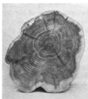
FIG. 69. Transverse section of yew, showing annual rings. Longest diameter, 5\frac{1}{2} ''; shortest, 4\frac{1}{8} ''; number of rings, 51. It will be noticed that the section is excentric; this is due to irregular growth.
