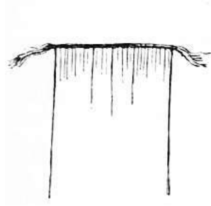
FIG. 10.—Section of back of book sewn on bands.
