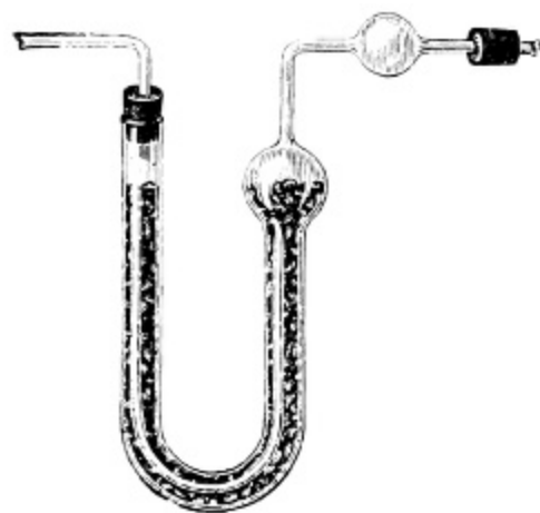
FIG. 41.—Tube for the absorption of carbonic acid. A plug of cotton
