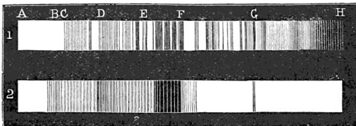
FIG. 74.—Absorption spectra of nitrogen dioxide and iodine.
