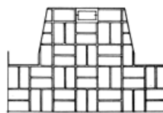
Fig. 39. Hearth With Brick Flat
