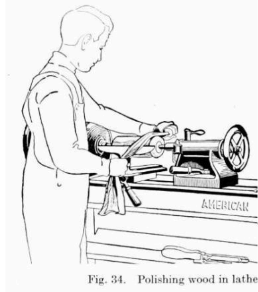
Fig. 34. Polishing wood in lathe
