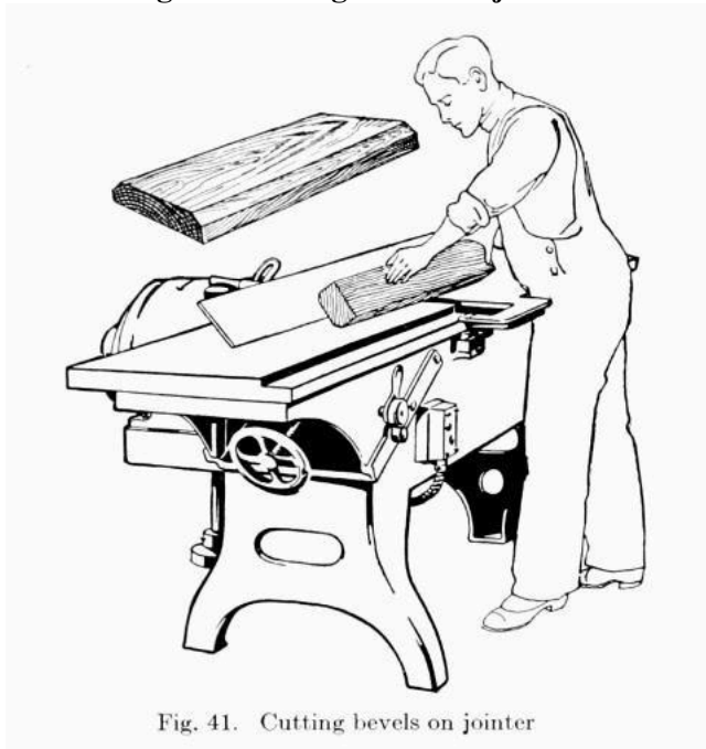
Fig. 41. Cutting bevels on jointer
