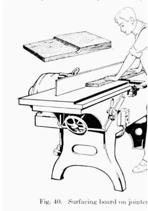
Fig. 40. Surfacing board on jo
