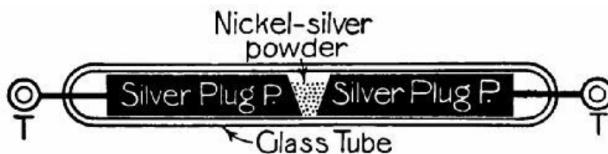
FIG. 60.—A Marconi coherer.
