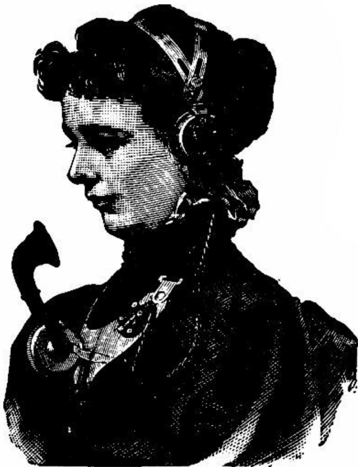
FIG. 65.—The headdress of an operator at a telephone exchange. The receiver is fastened over one ear, and the transmitter to the chest.
