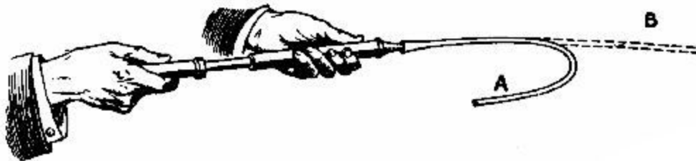
FIG. 13.—Showing the principle of the steam-gauge.
