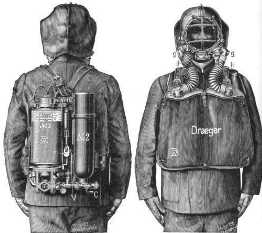
FIG. 38.—Showing the Potash Cartridge No. 2 with Change Mechanism X; No. 2 Oxygen Cylinder with Spanner V; and on the Left a Hexagonal Socket U, for unscrewing the Locking Nuts of Reserve Cylinders ( R. Jacobson )
