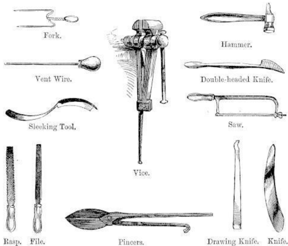
Fork. Vent Wire. Sleeking Tool. Rasp. File. Vice. Pincers. Hammer. Double-headed Knife. Saw. Drawing Knife. Knife.
