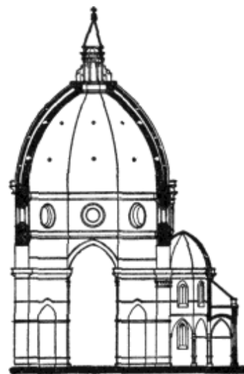
FIG. 159.—SECTION OF DOME OF DUOMO, FLORENCE.
