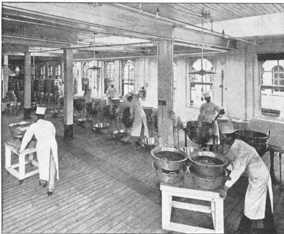
FIG. 32. —Preserving kettles in a large factory. Courtesy of H. J. Heinz Co.
