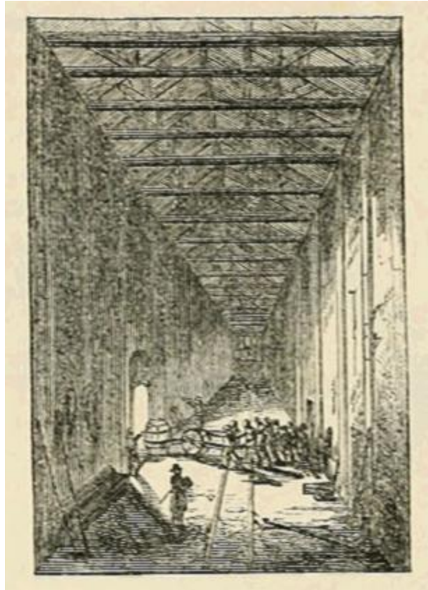
PLATE GLASS CASTING. BRINGING OUT THE POT.
