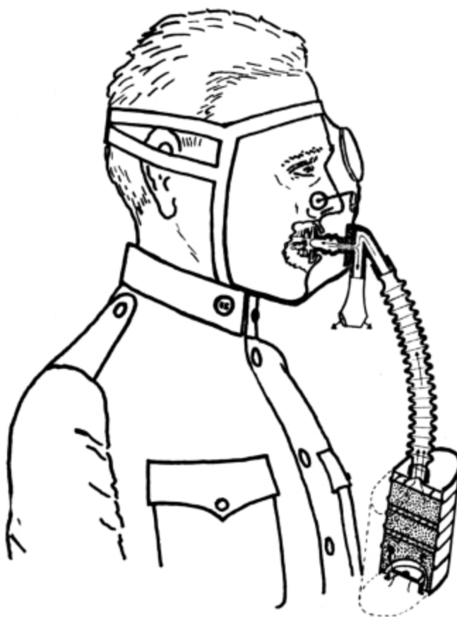
FIG. 53.—Diagrammatic Sketch of Box Respirator Type Mask.
