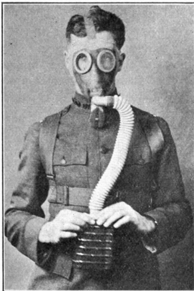
FIG. 66.—Ammonia Mask, Showing Relative Size of Canister.
