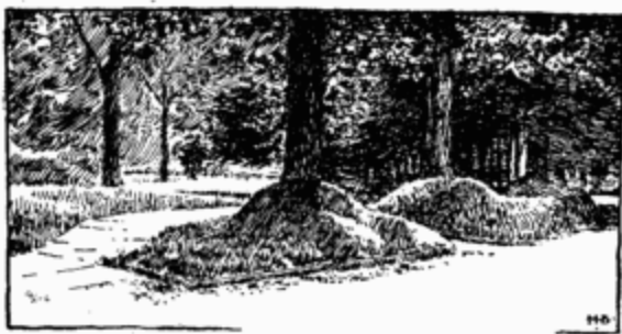
173. A method of saving valuable trees along streets on which heavy lowering of grade has been made.
