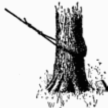
170. The wrong way of attaching a guy rope.
