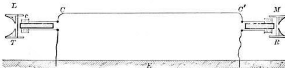
FIG. 241.—Diagram of a simple telephone circuit.
