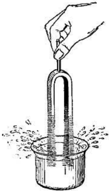
FIG. 164.—Sprays of water show that the fork is in motion.
