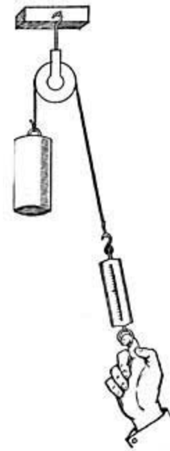
FIG. 109.—By means of a pulley, a force in one direction produces motion in the opposite direction.
