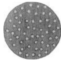
SECTION OF THE GRAPPLING LINE.
